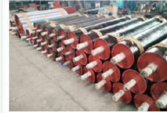
Conveyor Take Up Pulley
