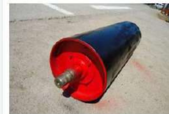
Conveyor Bend Pulley
