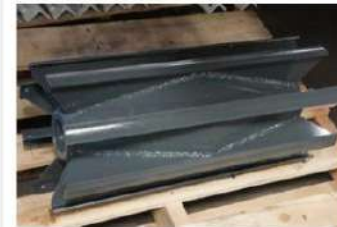
Conveyor Wing Pulley
