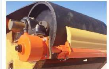
Conveyor Head Pulley
